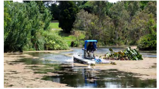
Steven Liu picking up floating aquatic vegetation in the new amphibious harvester machine in the Ornamental Lake at Melbourne Gardens Photo: Ricardo Simao
